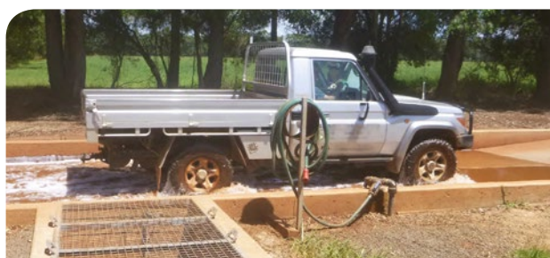
An automatic vehicle wash down bay that provides protection against soil borne diseases.
